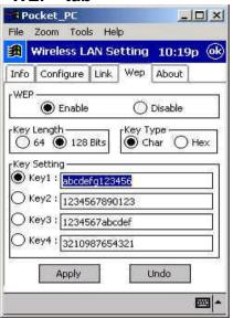
If an additional measure of security is desired on the wireless network, WEP (Wired Equivalent Privacy) encryption can be enabled. Please select "Enable" in the above screen, if you wish to activate encryption.
